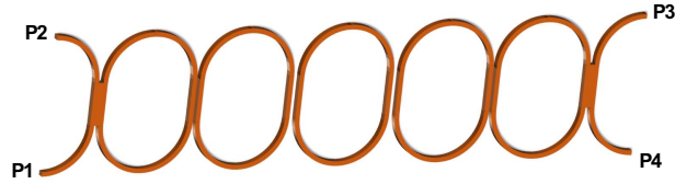
Fig. 13. Example B. The structure of the five-ring resonator filter.
