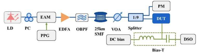
Fig. 5. Measurement setup for the fiber-optic link experiments
