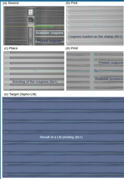
LNO 8 array printing Alignment accuracy < 500nm
