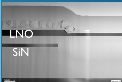
Patterned LNO printed on SiPho wafer
