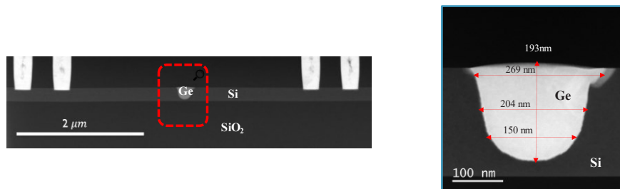
Fig. 1. TEM images of the Ge/Si PD showing the deeply recessed Ge inside the silicon
