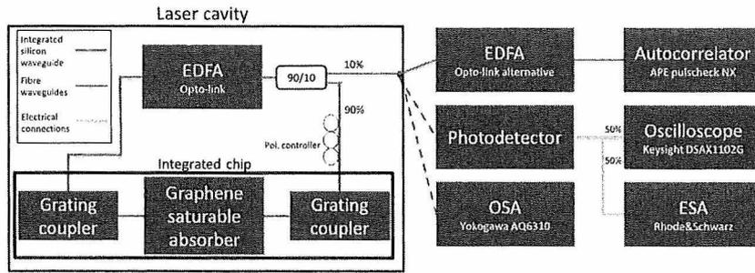
Fig. 2: Schematic of the experimental setup. The section in the black box indicates the laser cavity, and the section on the right the measurement equipment used
