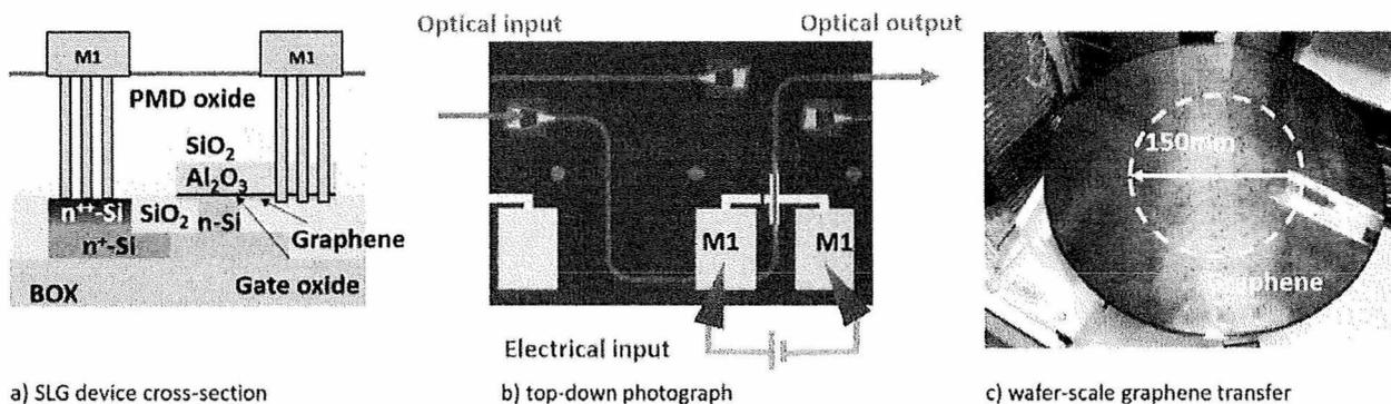
Fig. 1: The graphene saturable absorber assembly used for passive mode-locking [19]. Figure a) shows the schematic cross-section of the graphene modulator, Figure b) shows a top-down photograph of the device used as a saturable absorber. And Figure c) shows the 300mm patterned silicon wafer on which a 6 inch graphene sheet is placed.
