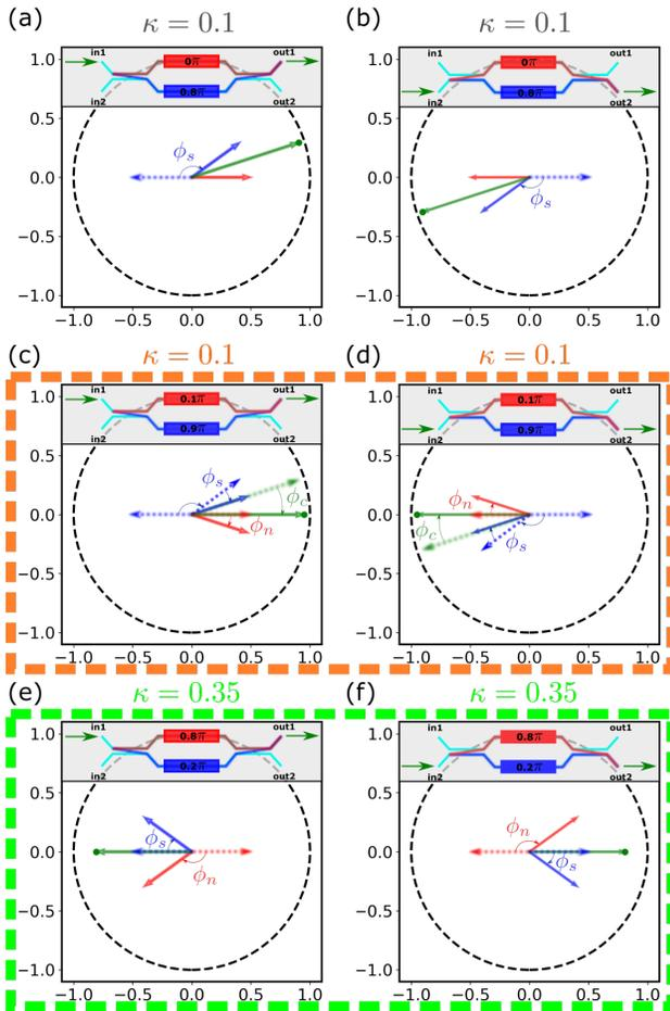
Fig. 2. Decomposition of the complex amplitude into two phase vectors (phasors) representing the North and South arm in a tunable MZI. The North arm is represented in red, and the South arm in blue. (a,c,e) illustrate the case where light travels from in1 to out1; while (b,d,f) show the transmission from in2 to out2. The coherent combination of these two beams gives us the amplitude vector in green which as the sum of the red and blue phasors.
