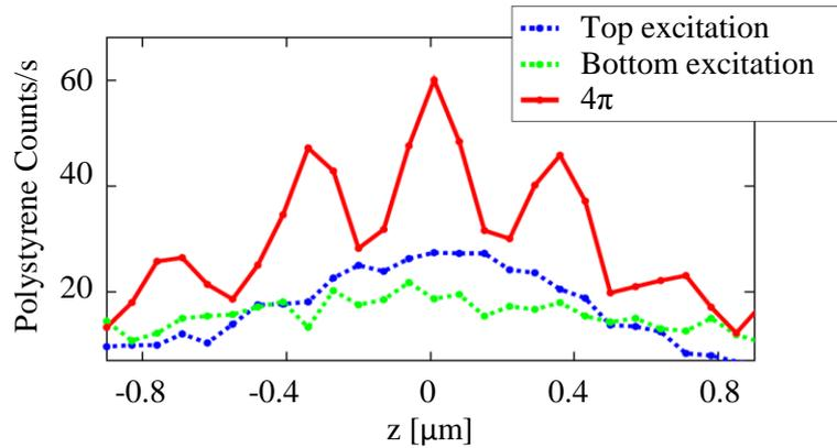
**Fig.5.** Standard confocal and  $4\pi$  point spread functions in the axial direction.
