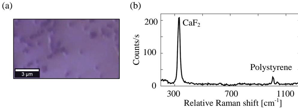
**Fig.3.** Polystyrene nanoparticles of 250 nm diameter. (a) Visible image. (b) Raman spectrum. The  $\text{CaF}_2$  peak comes from the substrate and the polystyrene peak around  $333 \text{ cm}^{-1}$  corresponds to the particles.
