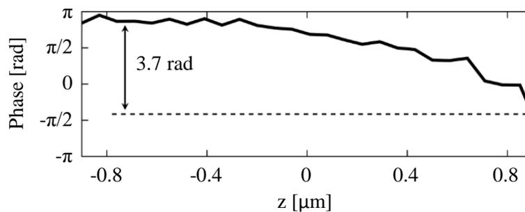
**Fig.4.** Phase shift needed between top and bottom beams to maximize the Raman polystyrene peak.
