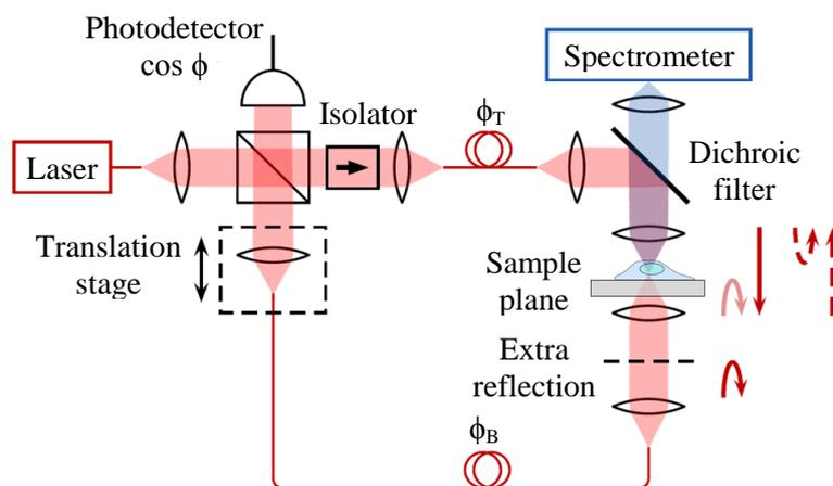
**Fig.2.** Optical schematic of the  $4\pi$  Raman microscope used in the experiments. Red arrows indicate different beams travelling through the setup. Dashed arrows are filtered out by the isolator. The extra reflection is optional, depending upon the strength of the sample plane reflection in light red.
