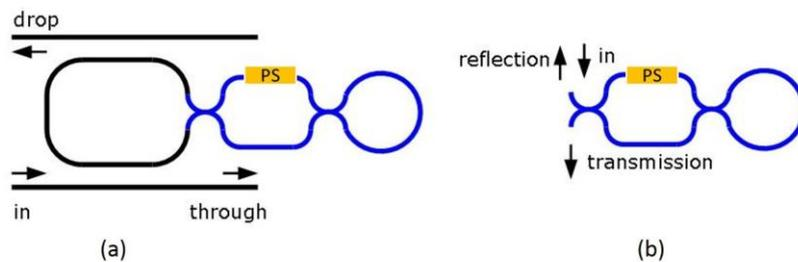
**Fig. 2.** (a) Schematic of our device and (b) the reflector, respectively. PS refers to a phase shifter.
