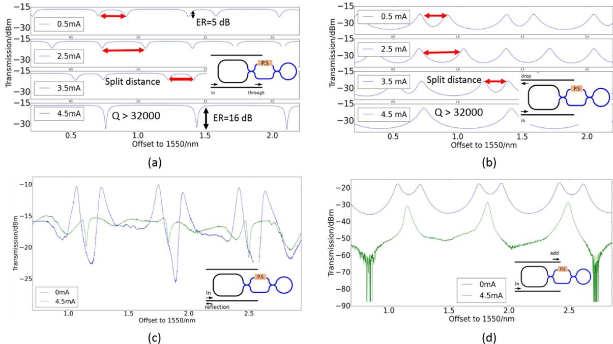
**Fig. 1.** Measured spectra of (a) through port, (b) drop port, (c) reflection and (d) add port under different tuning current. With the proper phase change, resonance splitting at through and drop port is eliminated, giving a higher extinction ratio. Besides, the reflection to *in* port and leakage to *add* port can be dramatically suppressed. PS means a phase shifter.
