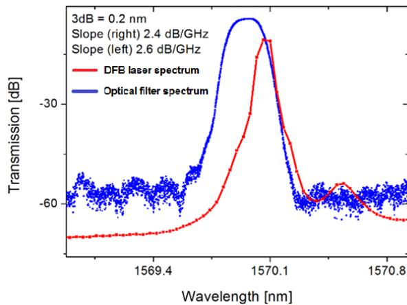
Figure 3: Optical spectrum of the laser with respect to the filter transmission spectrum.
