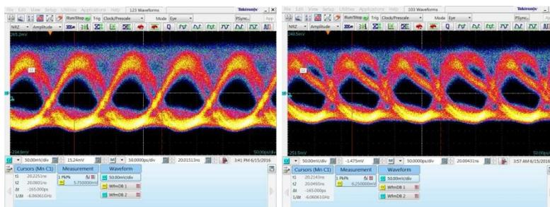
Figure 4. Eye diagrams at 10 Gb/s for the back-to-back case and after transmission over 20 km SSMF.
