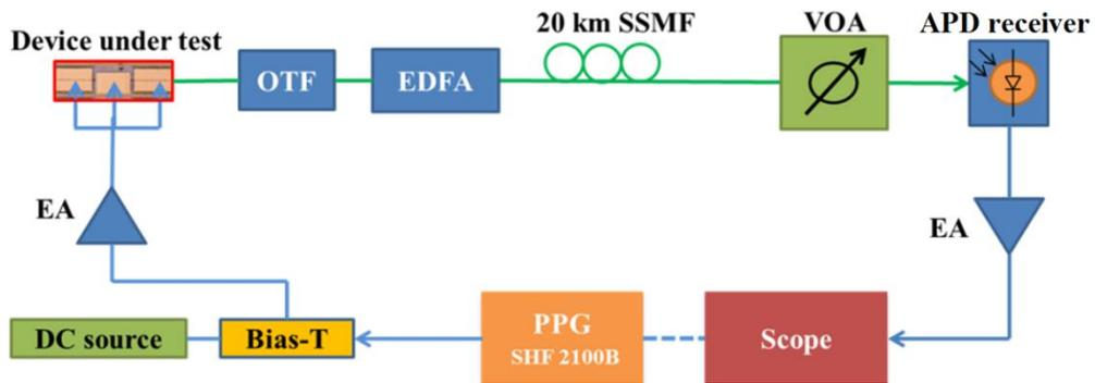
Figure 2: Schematic of the large signal measurement set-up for the 10G-PON measurement.
