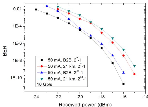
Figure 5: BER vs received optical power at 10 Gb/s for two different PRBS patterns lengths and for a 50 mA bias current to the DFB laser.
