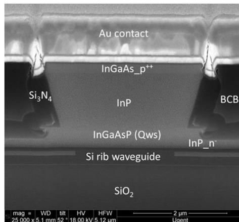
Figure 1: SEM picture of the cross section of a fabricated device
