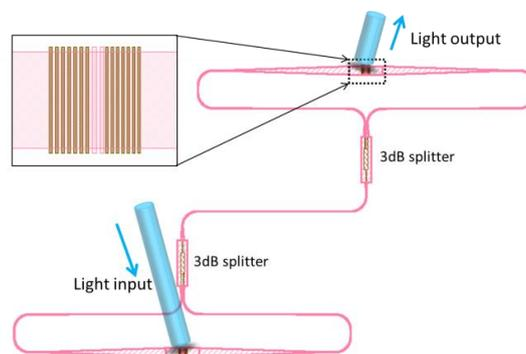
**Figure 3.** The test structure for the two-way-fed grating couplers.
