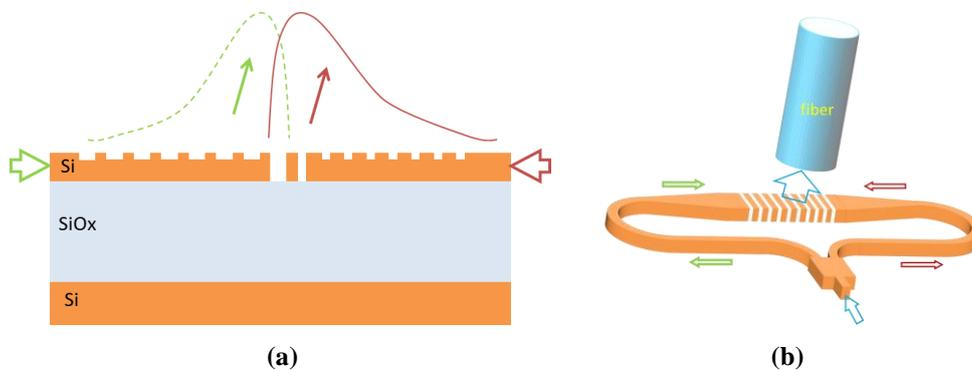
**Figure 1.** (a) Cross-section of a double grating. The green and red arrows show the directions of the input light beams from the waveguides and the light beam coupled to free space. The green and red curves on top of the grating region show the designed electric field profile of the output light beams. (b) 3D schematic show of the TWF-GC: including a double-grating and a 3dB coupler.
