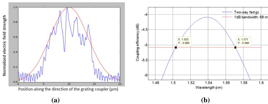
**Figure 2.** (a) Simulated electric field profile of the out-coupled field on top of the TWF-GC (blue line) and the mode profile of the single mode fiber (red line). (b) Simulated coupling spectrum of the TWF-GC to a single mode fiber, where the 1dB bandwidth is around 68 nm.
