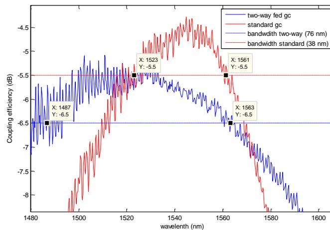
**Figure 4.** The measured transmission spectra of the fabricated two-way fed grating coupler (blue) and the standard grating coupler (red).
