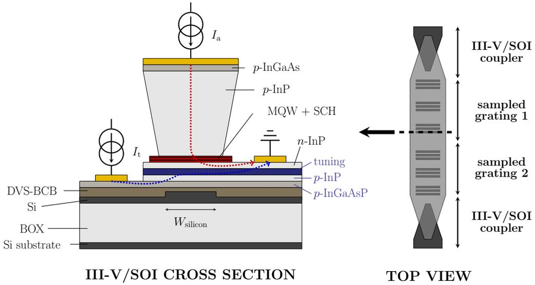
Figure 1: Layout of the proposed III-V/SOI TTG laser diode.  $I_a$  and  $I_t$  represent the active and tuning current respectively.
