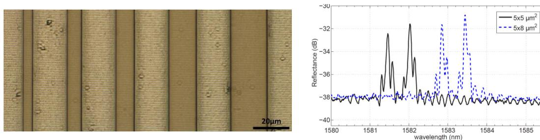
Fig. 3. (left) Microscope image of 5  $\mu\text{m}$ , 8  $\mu\text{m}$ , 10  $\mu\text{m}$ , 15  $\mu\text{m}$ , 20  $\mu\text{m}$  wide waveguides (5  $\mu\text{m}$  thick) patterned on top of grating structures inscribed in the cladding layer. (right) Reflection spectrum of the 5  $\mu\text{m}$  and 8  $\mu\text{m}$  single mode waveguides, normalized to the source spectrum.
