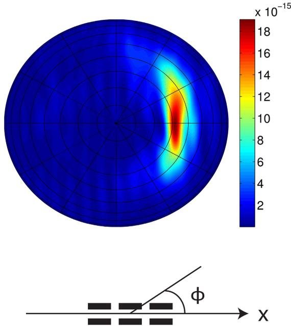
Fig. 3. Simulated far-field response on the hemisphere above the grating. The center of the grating coincides with the origin of the coordinate system, as indicated by the schematic top view. Concentric circles represent increments of  $10^\circ$  in the polar angle  $\theta$ , while radial lines correspond to steps of  $30^\circ$  in the azimuthal angle  $\phi$ . The highest intensity optical field is found around the direction  $\theta = 30^\circ$ ,  $\phi = 0^\circ$ .
