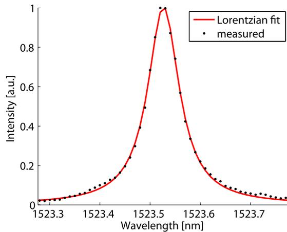
Fig. 6. Microring spectrum and resulting Lorentzian fit obtained by recording the near-vertical emission of the grating using an infrared camera.
