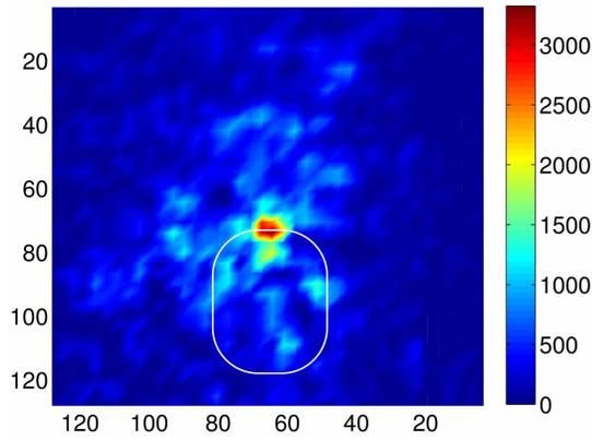
Fig. 5. Schematic microring and weak grating image as recorded by an infrared camera picking up the emission at  $30^\circ$ . Axes are expressed in  $\mu\text{m}$ . The color scale represents the counts per individual pixel.
