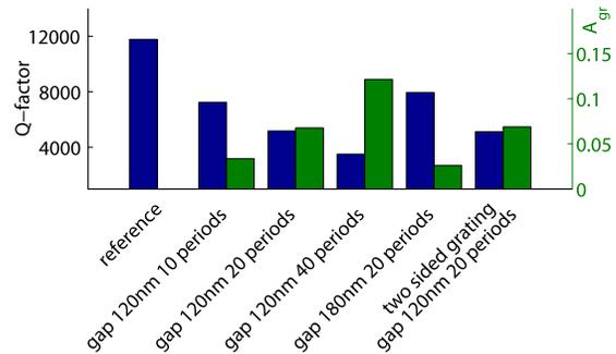
Fig. 2. Simulated quality factors and grating associated losses for microring resonators with different grating configurations.
