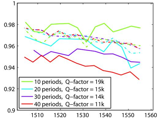
Fig. 4. Device and wavelength dependent coupling and round-trip loss for microrings with different number of weak grating periods. Dashed lines represent the coupling coefficient  $r$  while the full lines show the round-trip amplitude reduction coefficient  $a$ . The weak grating periods are 547 nm with 50% filling factor while the waveguide-grating gap is 130 nm.
