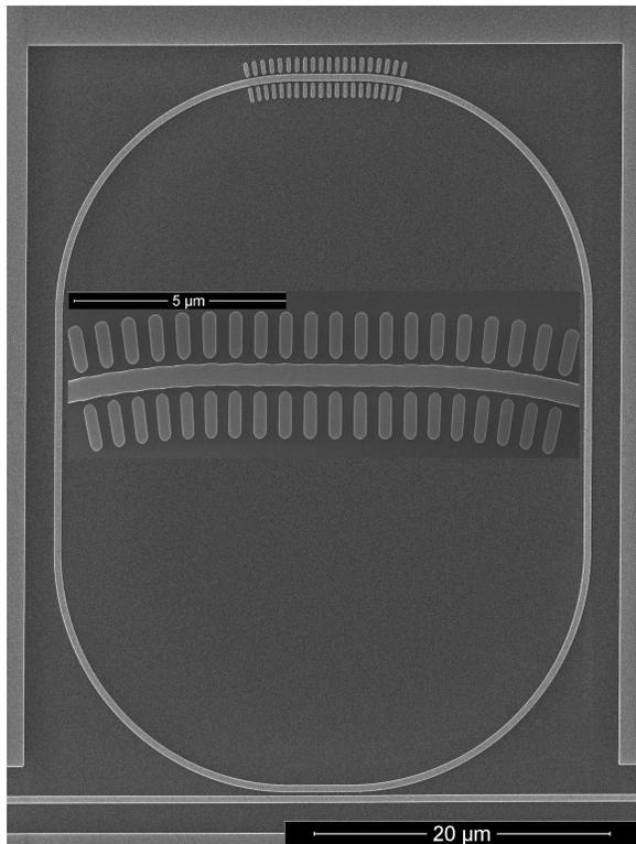
Fig. 1. SEM-picture of the microring resonator with weak grating in the vicinity of the waveguide. The inset shows a magnification of the grating region.
