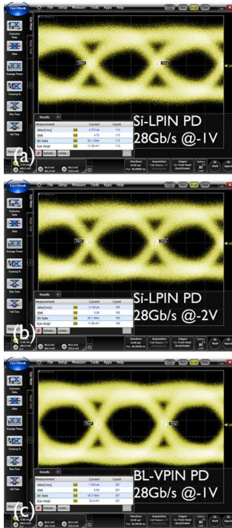
Fig. 9. 28 Gb/s eye diagrams of a Si-LPIN photodetector at (a) -1 and (b) -2 V. (c) 28 Gb/s eye diagram of a BL-VPIN photodetector at -1V.
