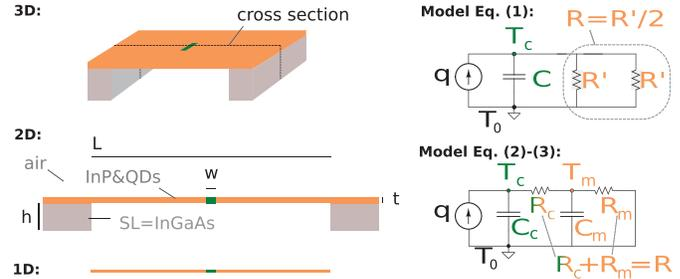
Fig. 1. A reduction of the geometry of a PhC cavity on a suspended membrane, to the principal dimension in which the heat flow takes place, gives rise to simple lumped circuit models. Incorporating the membrane temperature  $T_m$  in the model improves the description of the dynamics.
