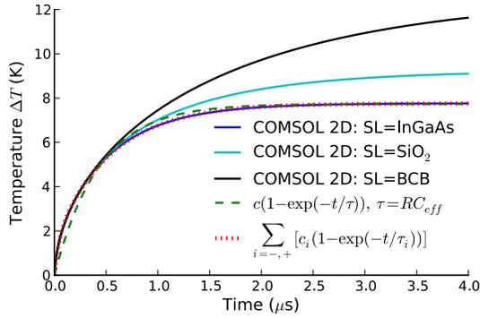
Fig. 3. The extended lumped circuit model (red dotted line) still explains the 2D simulation of the heat response of a PhC cavity (blue solid line) better than the fit of a single rising exponential (green dashed line). The choice for InGaAs in the sacrificial layer (SL) instead of, e.g., SiO<sub>2</sub> (solid cyan line) or BCB (solid black line), clearly influences the dynamics. The parameters used in this simulation can be found in Table I.
