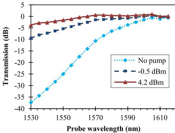
Fig. 5. Transmission spectrum of a 150  $\mu\text{m}$  long MIPS with 8 nm InGaAs quantum wells. The given pump power is the on-chip power calculated from transmission data through a reference waveguide.
