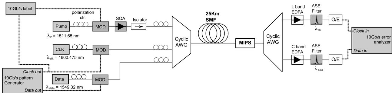
Fig. 6. Setup for the proof-of-principle clock distribution experiment.
