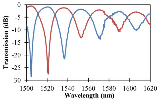
Fig. 2. Cross and through transmission of the 1x2 MZI.
