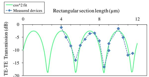
Figure 2. Demonstration of the device's polarization conversion behavior
