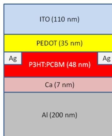
Fig. 2. Cross section of OSC with Ag grating integrated inside active layer
