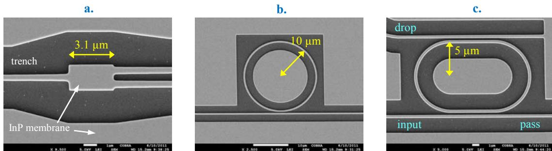
**Fig. 2 An MMI power splitter (a.), a ring resonator (b.) and a racetrack (c.) fabricated using IMOS post-bonding processing**
