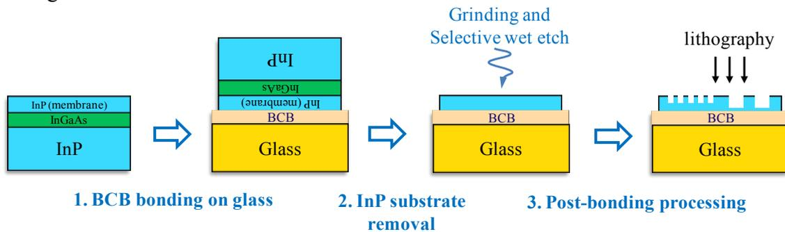
**Fig. 1 IMOS post-bonding fabrication scheme (not to scale)**
