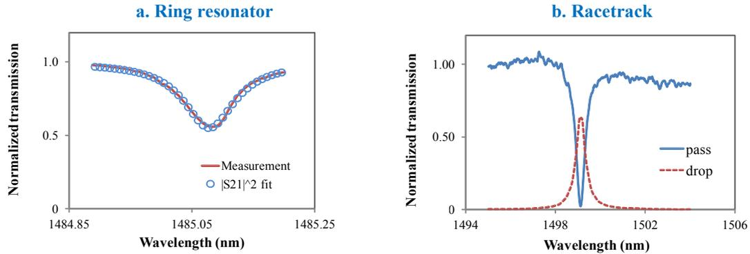
**Fig. 3 Measured transmission of the ring resonator (a.) and racetrack (b.) pictured in Fig. 2**
