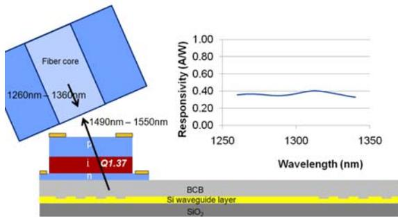
Fig. 2. Schematic cross-section of the realized photodetector for FTTH central office applications. In the inset, the experimentally obtained responsivity is plotted.
