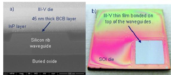
Fig. 1. Cross-section of a III-V on silicon layer stack and a top view image of a III-V epitaxial layer transferred to a silicon waveguide circuit
