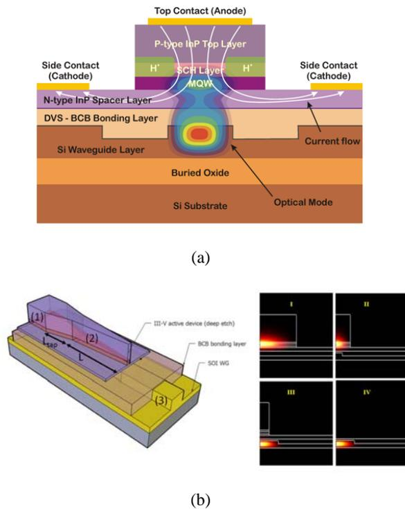
Fig. 3. Schematic cross-sections of the laser architectures
