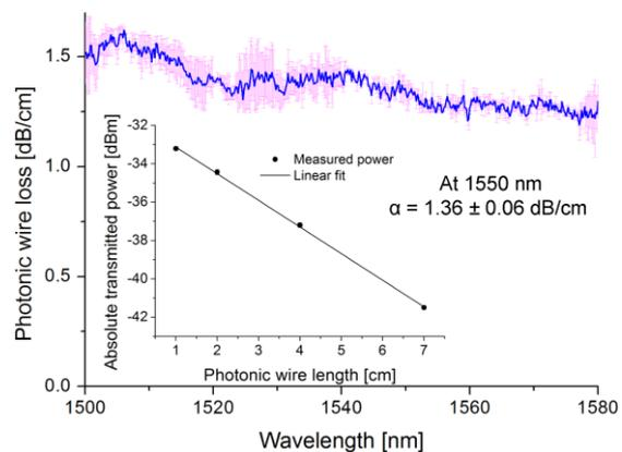
Fig. 4. Propagation loss of a photonic wire of 460 nm wide and 220 nm high.
