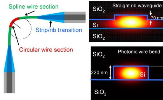
Fig. 1. Schematic of the implemented waveguide circuit with shallow-ridge straight section and deep etched photonic wire bends with the fundamental mode profiles.
