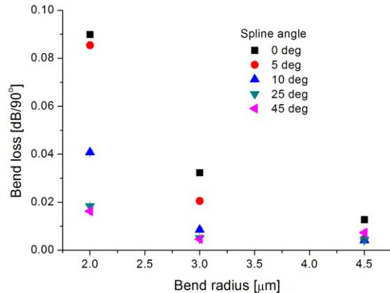
Fig. 3. Bend loss of photonic wires (460x220nm) with 5μm bend radius for different spline angles.
