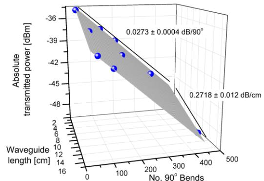
Fig. 2. Propagation loss and bend loss extraction from the fitting a 2D plane to the measured
