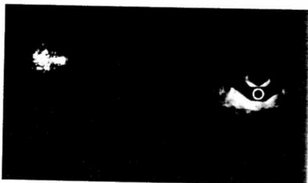
Figure 2: IR image of lasing of \Phi 40\mu\text{m} disk laser coupled to a waveguide. The light is output via a surface grating coupler.
