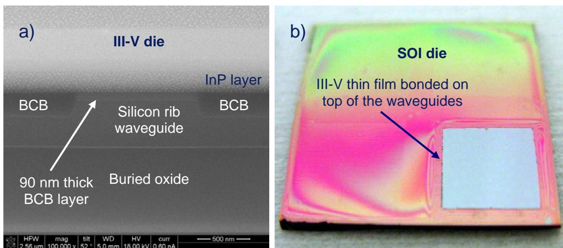
Figure 5. Impact of adhesion promoter AP3000 on the bonding test results: a) BCB layer thickness increased to 90 nm (using 1:3 BCB:mesitylene solution); b) peeling of III-V film is minimized during wet etching, resulting in clear and sharp III-V film edges.
