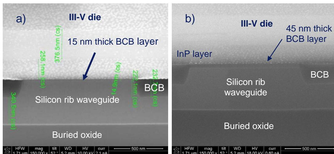
Figure 4. SEM images of ultra-thin BCB bonding layers on top of silicon waveguides: a) 15nm-thick layer, obtained using 1:7 BCB:mesitylene solution; b) 45nm-thick layer, produced by 1:3 BCB:mesitylene solution.
