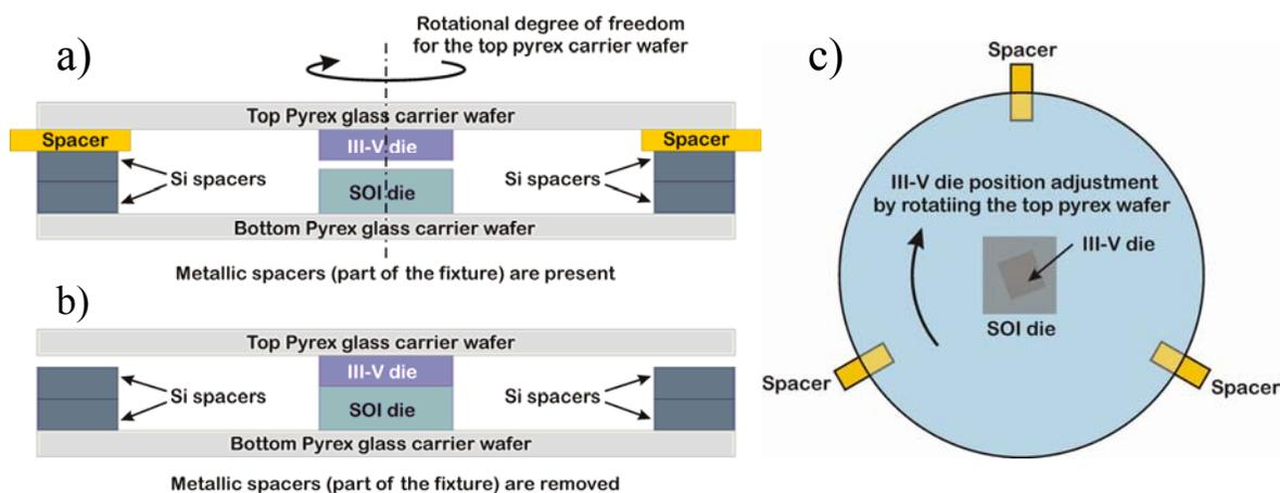
Figure 2. Die-to-die bonding setup: a) cross-section of the setup with spacers still in place – prior to bonding; b) cross-section of the setup after the spacers are retracted – III-V and SOI dies come into contact; c) top view of the setup – rotational degree of freedom enables easy positioning of a III-V die.
