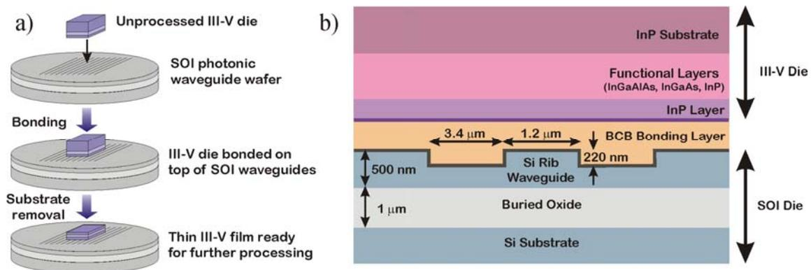
Figure 1. a) Heterogeneous integration of a III-V die on top of SOI waveguides based on bonding; b) Layout of our silicon rib waveguide structure with a III-V die comprising InGaAlAs active layers bonded on top of it.
