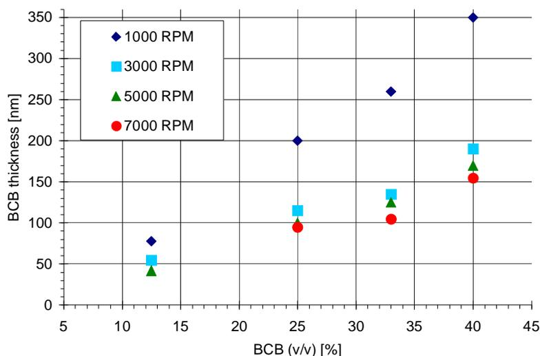
Figure 3. Thickness of cured BCB films, spin-coated on flat InP dies, depending on BCB volume ratio in BCB:mesitylene solution and rotation speed during spin-coating.
