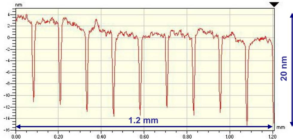
Figure 6. BCB surface profile perpendicular to SOI waveguides. Notches are observed at the locations of SOI waveguides, at 250  $\mu\text{m}$  pitch.
