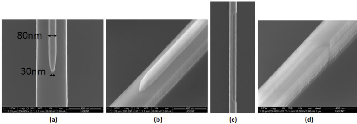
Fig. 2: SEM pictures: Vertical Taper tip (a,b) and Polarization Rotator (c,d).
