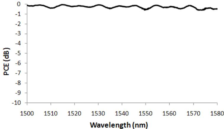
Fig. 3: Polarization Conversion Efficiency (PCE) measurement.
