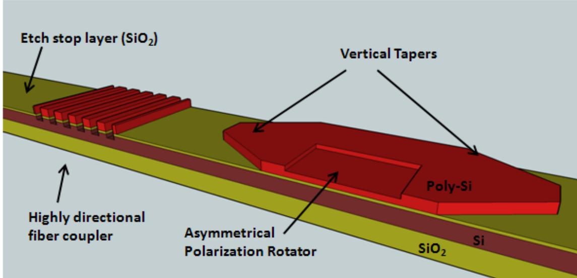
Fig. 1: Artist's impression of a highly directional fiber coupler and asymmetrical polarization rotator fabricated within the same process flow. (Dimensions are not to scale)
