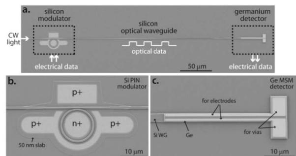
Fig. 3 Optical link with off-chip source, silicon modulator and germanium detector (from [19]).
