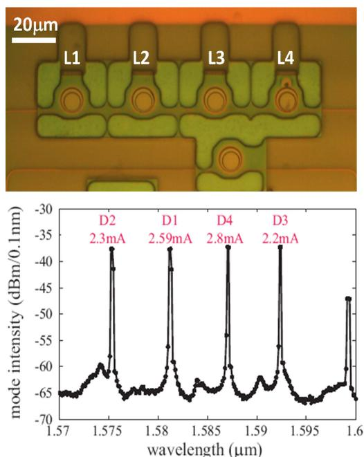
Fig. 4 Fabricated multiwavelength laser before metallization, composed of four MDLs on a single silicon bus waveguide. Spectra of multiwavelength lasers with 6 nm are also shown. The bias current of each MDL is indicated on the corresponding lasing peak (from [23]).
