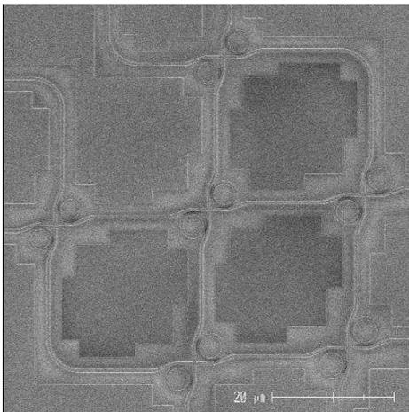
Fig. 2 Optical cross-connect (4x4) build up from individual resonator elements.
