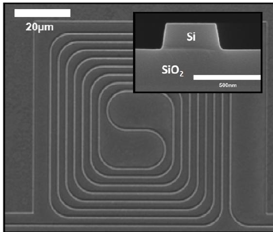
Fig. 1 Silicon on insulator photonic wire circuit (inset: waveguide cross section)(from [12]).
