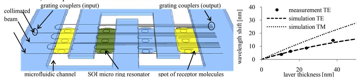
Fig. 1. A) illustration of the disposable lab-on-a-chip (not to scale), B) simulation and measurement of SiO<sub>2</sub> adlayers with increasing thickness.
