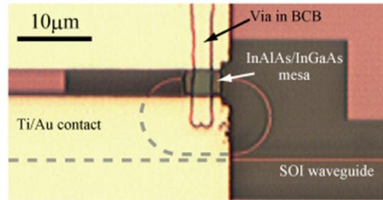
Fig. 3. Microscope image of resonant photodetector structure
