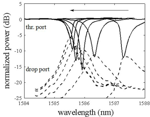
Fig. 2. Microdisk through port and drop port characteristics
