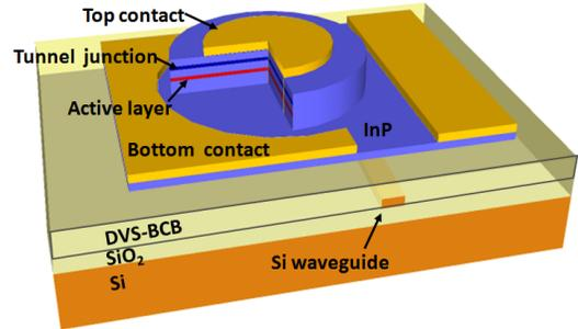
Fig. 1. Schematic representation of a heterogeneously integrated microdisk laser on SOI.
