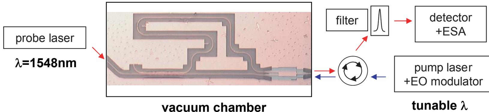
**probe laser light is detected and analyzed with electrical spectrum analyzer**
