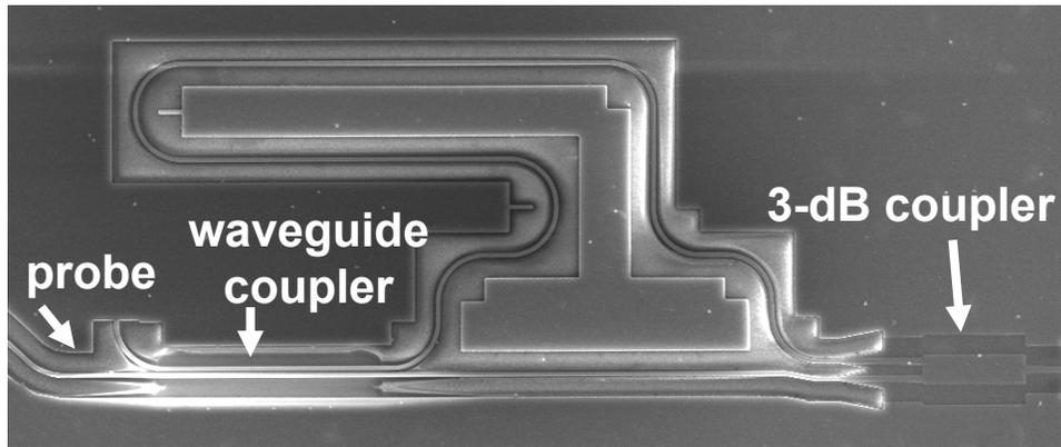
full device = unbalanced Mach-Zehnder Interferometer (delay length  $\Delta L$ ) with one MMI coupler and one waveguide coupler
