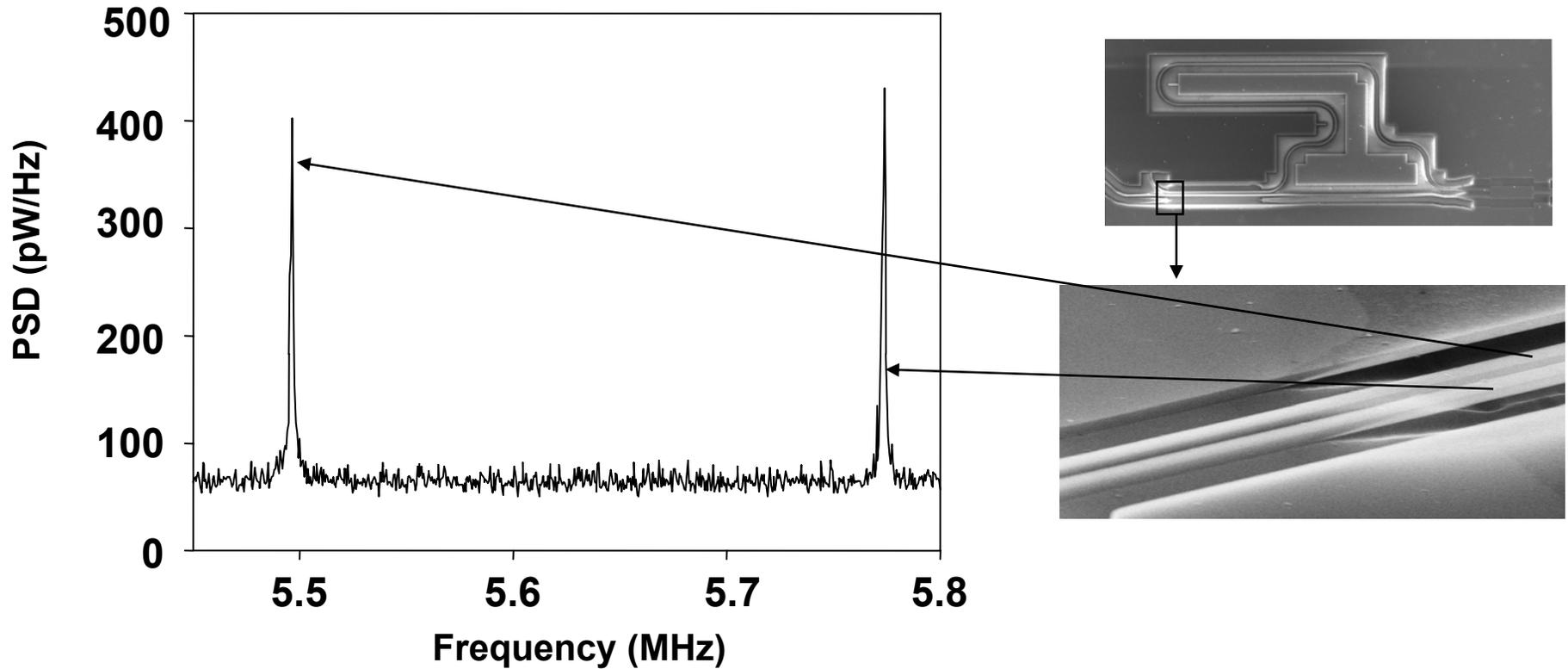
**Transduction (without pump) is measured/calibrated by recording thermal vibration noise (peak spectral density PSD)**
