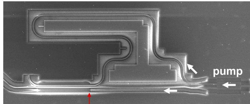
sweeping pump  $\lambda \Rightarrow$  fields arrive with different phase at waveguide coupler entrance
