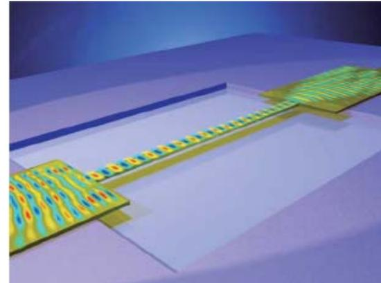
Experimental demonstration of *attractive* force between waveguide and substrate
