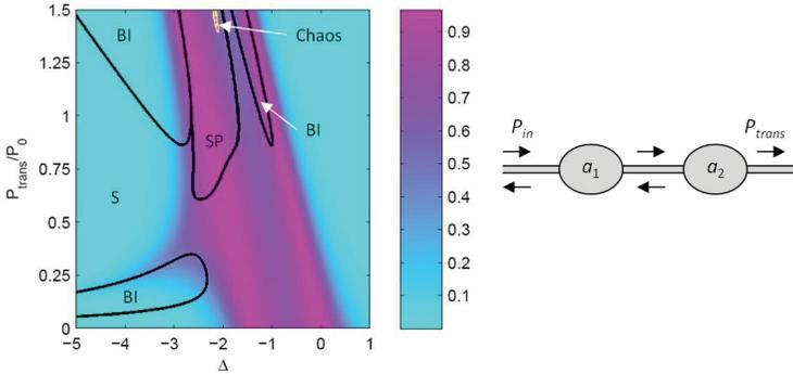
Figure: (left) Dynamical behaviour of two Kerr cavities. Transmitted power versus normalized detuning. The colorbar shows the transmission. (right) Schematic of the device
