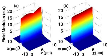
Fig. 1. (Color online) Intensity profiles along a tilted WG for (a) the standard and (b) the generalized rectangular wide-angle propagations.
