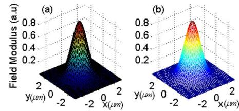
Fig. 3. (Color online) Magnitude of 3D Gaussian beam after propagating  $1 \mu\text{m}$  calculated by the generalized rectangular WA-BPM based on (a) DMI and (b) CJI.
