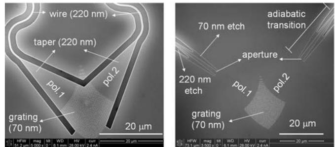
Figure 3. SEM-pictures of focusing 2D-grating couplers. (Left) Short non-adiabatic taper configuration. (Right) Shallow aperture configuration.
