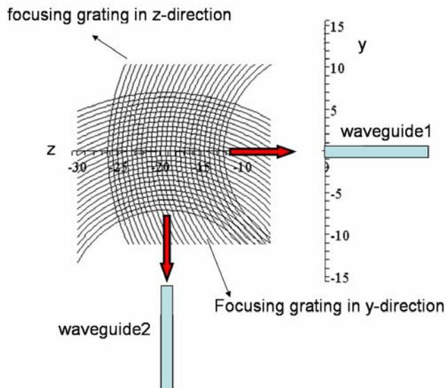
Figure 2. Overlay of two orthogonal 1D-focusing grating couplers.
