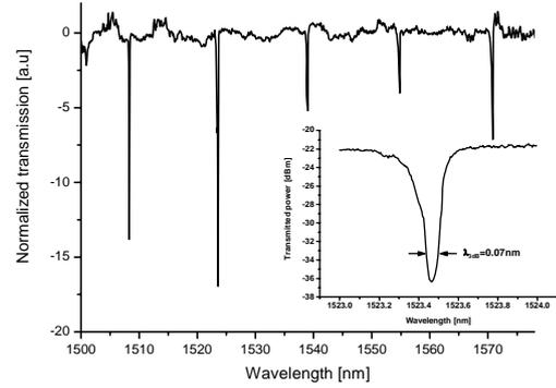
Figure 5. Transmission spectrum of the ring resonator
