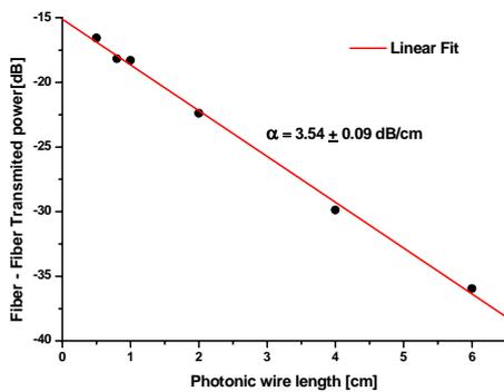
Figure 4. Transmitted power Vs Wire length at 1550nm
