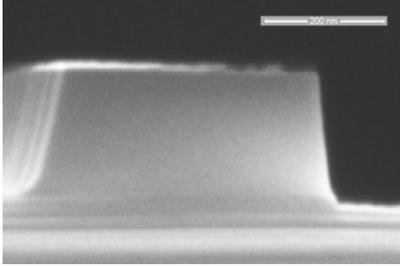
Figure 2. SEM image of an a-Si photonic wire
