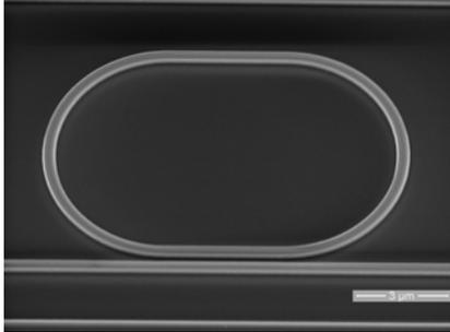
Figure 3. Race track ring resonator
