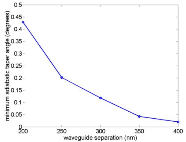
Fig. 5. Minimum adiabatic SOI taper angle versus waveguide separation for SOG bonding coupling scheme
