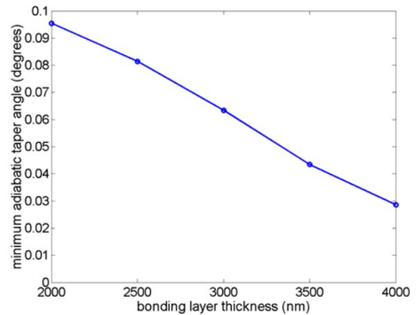
Fig. 8. Minimum adiabatic taper angle versus bonding layer thickness for BCB bonding coupling scheme
