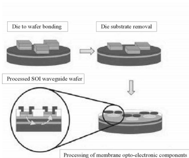
Fig. 1. Processing sequence for heterogeneous integration of III-V components and SOI waveguides
