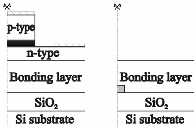
Fig. 2. InP membrane waveguide (left) and single mode high index contrast SOI waveguide (right).
