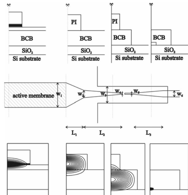
Fig. 6. BCB bonding coupling scheme - layout and mode transformation
