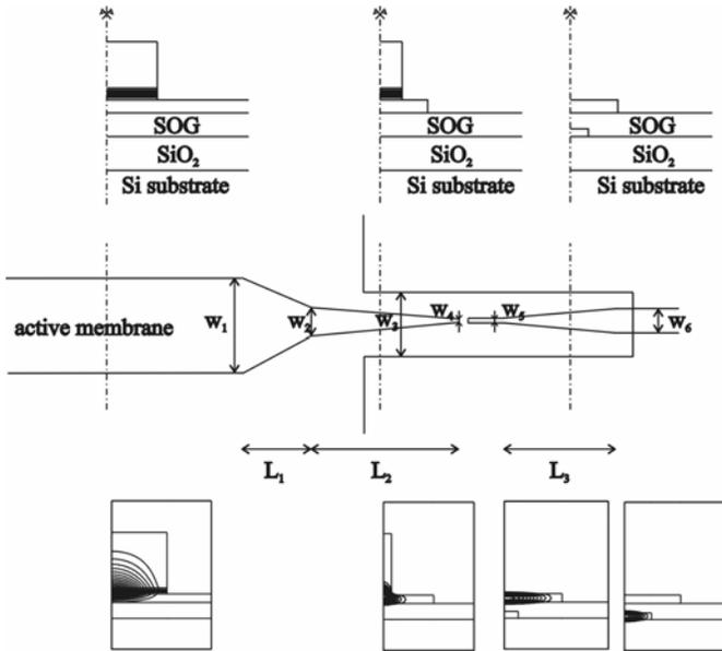
Fig. 3. SOG bonding coupling scheme – layout and mode transformation
