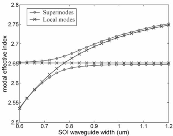
Fig. 4. SOI adiabatic taper operation principle – modal effective indices
