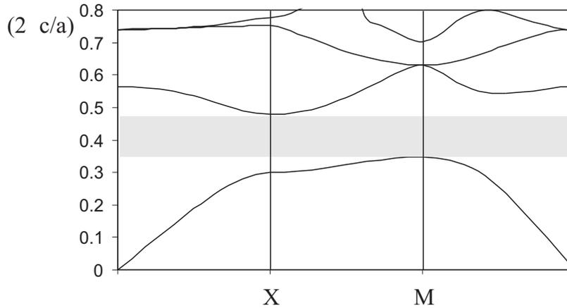
Fig. 1. The band-gap structure of the photonic crystal consisting of a square lattice of square dielectric rods ( $n = 3.4$ ) in an air background. The ratio of the side of the rods to the crystal period is  $d/a = 0.25$ .
