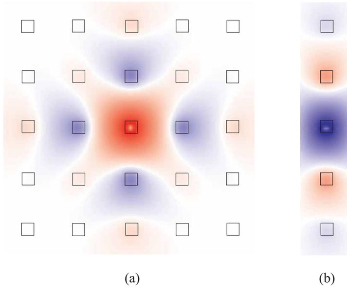
Fig. 3. (a) Photonic crystal geometry with Green's function at  $\omega = 0.38(2\pi c/a)$  superimposed. (b) Strip Green's function at  $\omega_{k_x} = 0.38(2\pi c/a)$  and  $k_x = 0.7\pi/a$  calculated using Eq. (6). In both cases  $\mathbf{r}_2 = 0$ .
