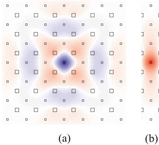
Fig. 6. (a) Diatomic photonic crystal geometry with Green's function at  $\omega = 0.4(2\pi c/a)$  superimposed. (b) Strip Green's function at  $\omega_{k_x} = 0.4(2\pi c/a)$  and  $k_x = 0.85\pi/a$ .
