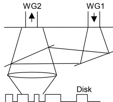
**Figure 2b: Far field approach with beam splitter**
