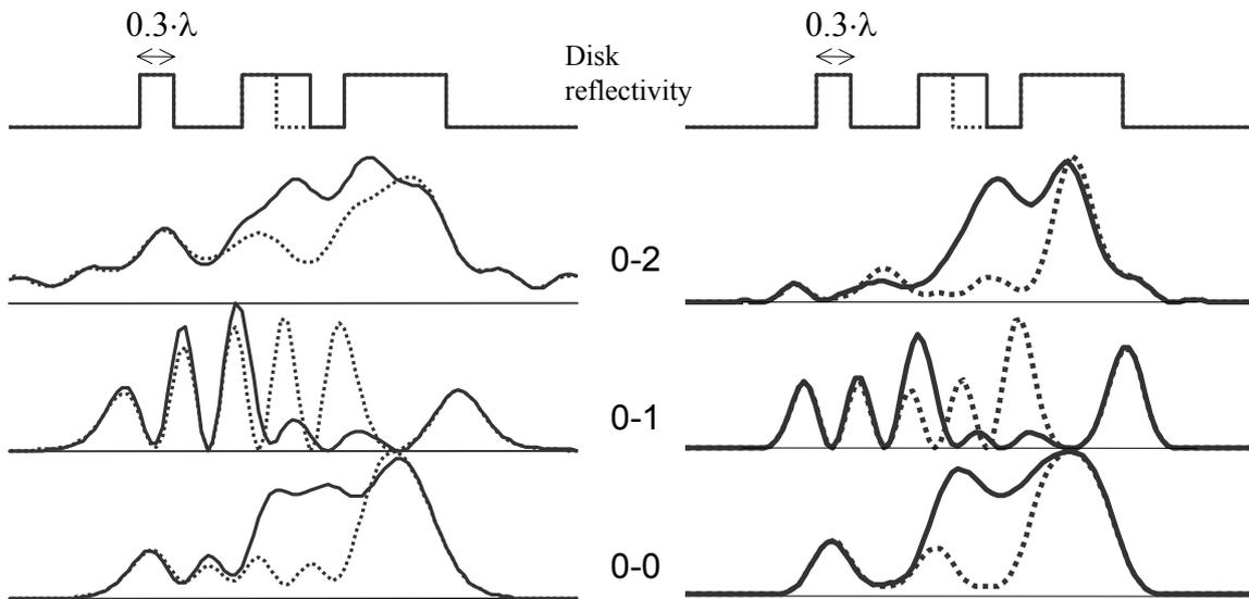
**Figure 3a: Bit pattern and mode-to-mode coupling curves in the intermediate field approach**
