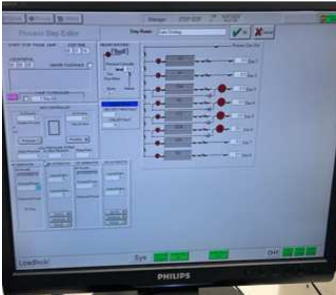
Figure A.2: ICP settings for etching GaAs/AlGaAs.
