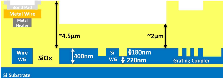
Figure 2.35: Schematics of the IMEC 400nm+ SOI cross-section with the integrated metal layers and back-end stack.
