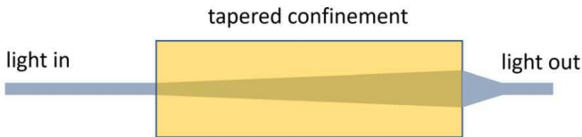
Figure 3.23: Schematic illustration of an alternative SOA design utilizing a tapered silicon waveguide. Transitions between the silicon and hybrid waveguides, which are not shown here, are designed to be adiabatic. At the output, the wider silicon waveguide is gradually tapered back to a single-mode waveguide [14].
