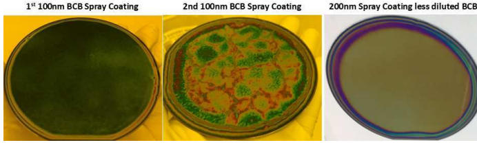
Figure 4.7: (Left) 1st layer of 100 nm BCB spray coated on a blank Si wafer, (Middle) 2nd layer of 100 nm BCB spray coated on the same wafer to reach 200 nm of BCB in total. (Right) One time of spray coating less diluted BCB on a blank Si wafer to reach 200 nm of thickness.
