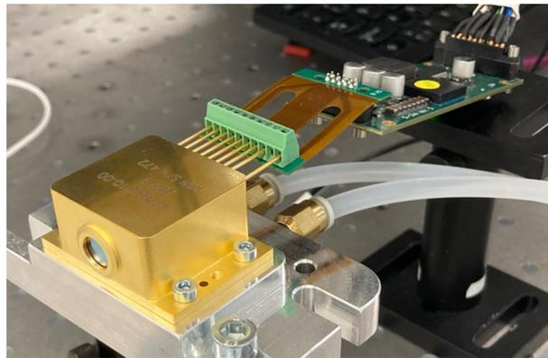
**Figure 11.** Fully packaged PIC in an HHL module connected to the S2-M driver.
