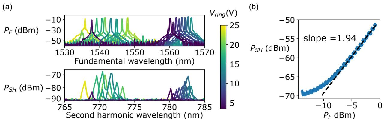
Fig. 2. (a) Thermal tuning of the laser using the Vernier resonance. Top: On-chip laser output power at the fundamental wavelength. Bottom: Second harmonic power at the detector for a sweep of the fundamental wavelength. (b) Power sweep on a test device with a 5 mm-long PPLN section using an external pump laser at 1595 nm showing quadratic dependency of the second harmonic power at the detector with respect to on-chip pump power.
