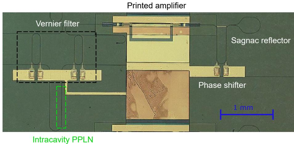
Fig. 1. Optical microscope image of the laser cavity. Using the Vernier effect, we can thermally tune the cavity resonance over a large frequency range. A section of the cavity is periodically poled to generate frequency doubled light.
