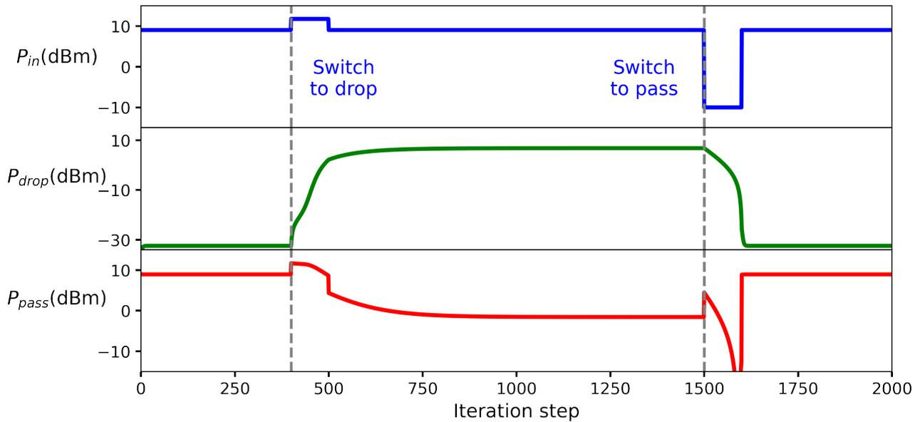
Fig. 2. (a) Dynamics of the saturable absorber based all-optical switch (parameters in Table I) using the modified transfer matrix method: first the input light is routed to the pass port, when applying a pulse at step 300 it is routed to the drop port and by removing the CW for a period at step 1500 it is routed back to the pass port. For the two states the extinction ratios are 30 dB and 10.1 dB and the insertion losses are 0.1 dB and 1.8 dB respectively
