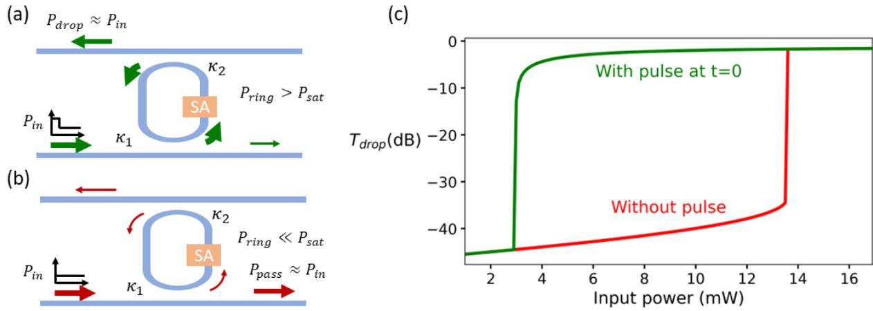
Fig. 1. (a) Schematic optical transmission from the input to the drop port of a continuous wave input with an initial pulse (b) without an initial pulse (c) Simulated power transmission to the drop port for (a) (green) and (b) (red) for a saturation power of 0.6 mW and optimized coupling coefficient and input power listed in Table I
