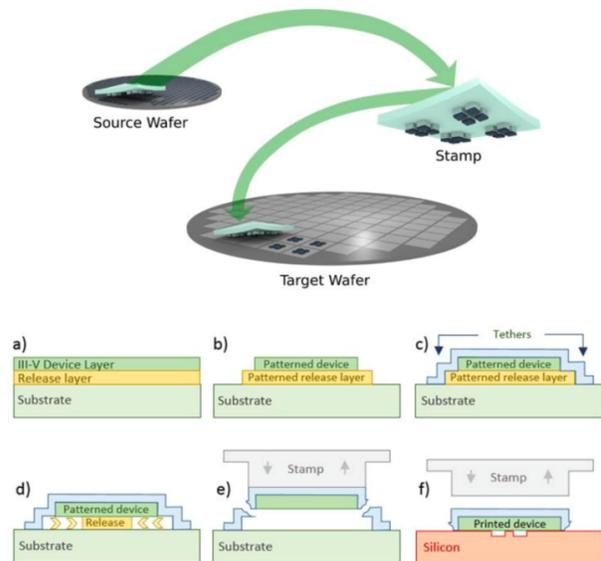
Fig. 3. (top) Micro-transfer printing uses a stamp to pick up devices from a source wafer and to print those devices on a target wafer. (bottom) By etching the release layer the processed and tested III-V devices are released from the source wafer and can be transferred to a target wafer.
