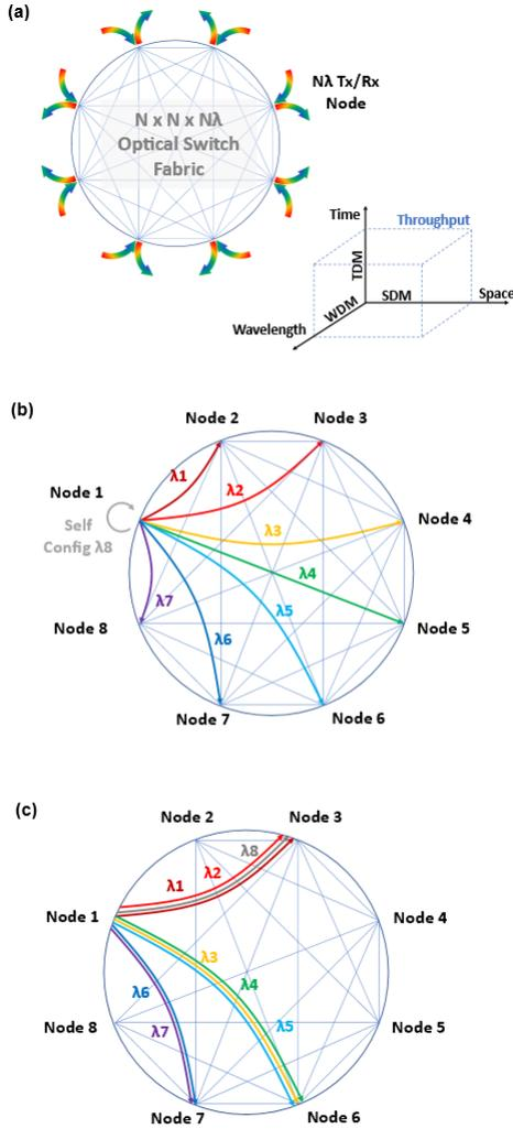
Fig. 1. (a) A conceptual figure of a fully non-blocking  $N \times N \times N\lambda$  optical switch fabric. (b) Illustration of all-to-all reconfigurable interconnection by allocating a wavelength to any pair of nodes. (c) Illustration of bandwidth steering by allocating multiple wavelength capacity between hot nodes in order to resolve congestion.
