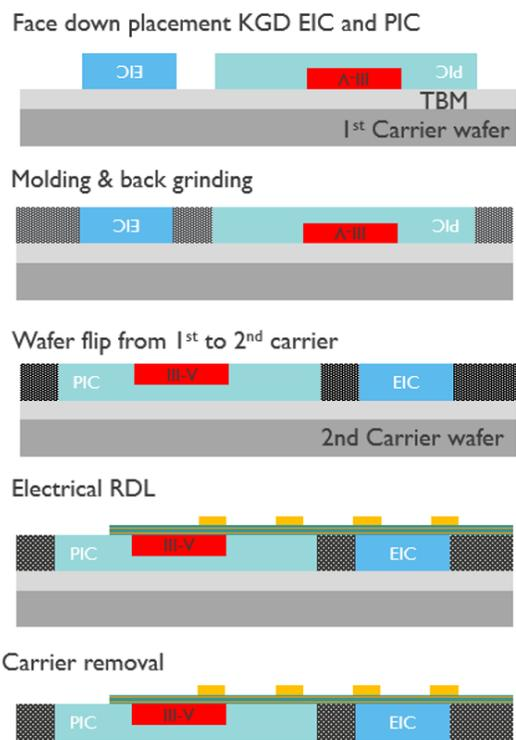
Fig. 4. PUNCH fan-out wafer-level packaging process flow for dense integration of PICs with EICs, enabled by the electrical redistribution layer.
