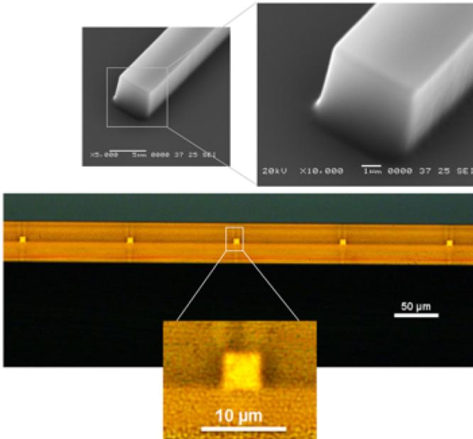
Fig. 5. Polymer waveguide based ORDL for interfacing different PICs and PICs with fiber arrays.
