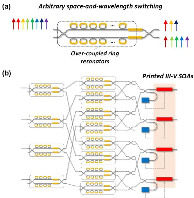
Fig. 2. (a) Proposed  $2 \times 2 \times 8\lambda$  SE with 8 pairs of MRR phase shifters. (b) A  $4 \times 4 \times 4\lambda$  dilated Banyan switch building block.
