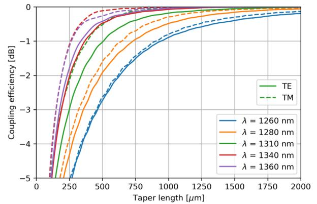
Fig. 6. Broadband behaviour of the adiabatic SiN-ORDL coupler, resulting from Lumerical Mode EME simulations.
