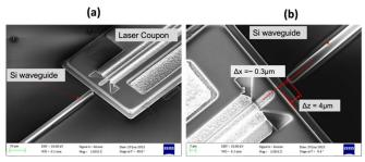
Fig. 12. (a) SEM image of a 1.5 mm long QD laser coupon placed in front of a 3 µm thick, deep-etched waveguide on SOI wafer. (b) Lateral and longitudinal alignment of laser with respect to the Si waveguide.
