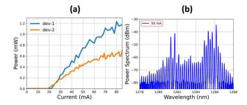
Fig. 14. (a) L-I characteristics measured with a broad area detector emerging from the 3  $\mu$ m thick waveguide. (b) The emission spectrum of the waveguide coupled light at 20 °C with 50 mA drive current.
