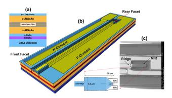
Fig. 3. (a) GaAs QD laser epitaxial structure grown by Innolume GmbH, (b) Laser coupon schematic showing the metal top contacts, ridge waveguide and mirror. (c) SEM image of a MIR mirror (6.5 μm wide and 50 μm long) and the inset shows a schematic of the MIR derivation from 1x2 MMI.
