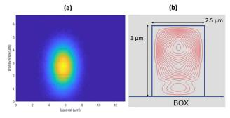
Fig. 15. (a) Measured near field beam profile at the exit of the 5 mm long Si waveguide. (b) Simulated electric field of the excited mode in the 2.5  $\mu$ m wide and 3  $\mu$ m thick Si waveguide when the vertical misalignment between laser and receiving waveguide is 0.67  $\mu$ m.
