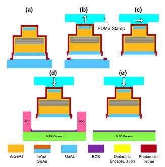
Fig. 6. Schematic sequence of picking and printing laser coupons onto target (a) Laser coupon ready for MTP, (b) Pick of the laser coupon with a PDMS stamp, (c) Transfer of coupon, (d) integration into a recess on SOI or (e) onto a planar surface.
