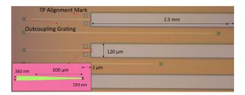
Fig. 9. Optical microscope image of the 7  $\mu$ m deep, 120  $\mu$ m wide and 2.5 mm long recesses defined in SOI. The inset shows the schematic of single tip Si waveguide inverse tapered from 150 nm to 380 nm over a 100  $\mu$ m distance. Waveguide tip is recessed from the etched facet by 2  $\mu$ m.
