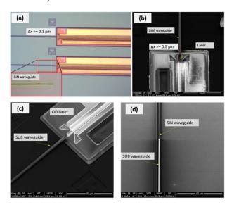
Fig. 16. (a) 1.8 mm long QD laser coupon transfer-printed on 70 nm BCB. The inset shows the SiN waveguide that starts from  $\sim\!\!10~\mu m$  away from the laser facet. (b) SEM image of a laser after SU-8 polymer waveguide definition. (c) Side view of a laser shows there is no gap between the laser facet and receiving SU-8 polymer waveguide. (d) SEM image of 1  $\mu m$  wide SiN waveguide and SU-8 waveguide termination tip.
