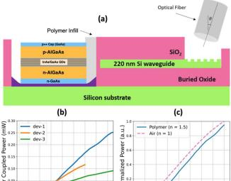
Fig. 11. (a) Schematic of coupling from a laser printed in SOI trench to 220 nm Si waveguide and then to single mode fiber through the out-coupling grating. (b) Fiber coupled power as a function of current for 3 devices. (c) L-I curve (for dev-1) shows the change in threshold current before and after the longitudinal gap is filled with an index matching polymer. The light intensity is normalized for better comparison.
