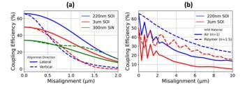
Fig. 2. Simulated coupling efficiencies as a function misalignment in lateral, vertical and longitudinal directions for fundamental TE mode transmission from a laser (2.5 μm ridge) to 220 nm SOI, 3 μm SOI and 300 nm SiN waveguide. (a) Horizontal (continuous line) and vertical (dashed line) misalignment, and (b) Longitudinal misalignment with air-gap (continuous line) or in-filled with polymer of n=1.5 (dashed line).
