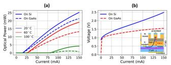
Fig. 8. (a) Temperature-dependent output power as a function of current for lasers with 2.5 μm-wide ridge and 1.5 mm cavity length on GaAs and after MTP onto Si with 70 nm BCB, and (b) V-I characteristics of lasers on GaAs and Si at 20°C. Electrical contact configuration and current path for lasers (inset).
