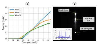
Fig. 18 (a) Measured L-I characteristics from 1.5 mm long laser coupons integrated with a SiN waveguide. Signal is first edge-coupled into 3  $\mu$ m wide and 2.2  $\mu$ m thick SU-8 waveguide, and then evanescently coupled to underlying SiN waveguide. The inset shows the spectrum of waveguide coupled light at 20°C. (b) Infra-red camera image of the laser and SiN when the laser is biased at 50 mA.
