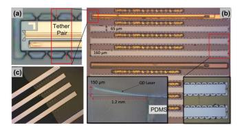
Fig. 4. (a) Photoresist tether defined with antiphase configuration on 65  $\mu$ m wide coupon. (b) Microscope image of coupon stub on GaAs substrate after the pick-up. Side view of a laser coupon picked-up by bulk PDMS and curled due to stress on coupon (left-inset), Image of the coupon stubs shows a clean undercut (right-inset), (c) Image of bottom surface of coupons after the release etch.
