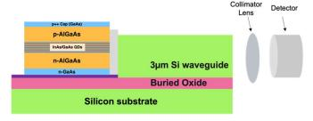
Fig. 13. Schematic of edge-coupling from a laser to 3  $\mu$ m thick Si waveguide and the coupling from the cleaved facet to a broad area detector.
