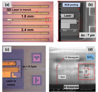
Fig. 10. (a) Images of 1.8 mm and 2.4 mm long QD laser coupons MTP into 7  $\mu$ m deep trenches on SOI with 100 nm spray-coated BCB. (b) SEM image of a coupon inside deep trench shows 7  $\mu$ m longitudinal spacing between laser and SOI facet due to BCB pooling at recess edge. (c) Detail of the lasing facet shows a lateral misalignment of  $\Delta x < 0.5 \mu$ m. (d) FIB cross section image near the Si waveguide tip shows the Si waveguide is 150 nm wide and 220 nm thick.
