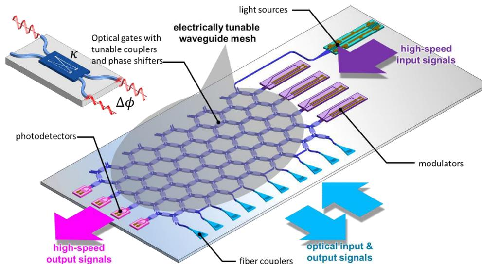
Fig. 1. Schematic illustration of a programmable photonic chip with a hexagonal waveguide mesh.
