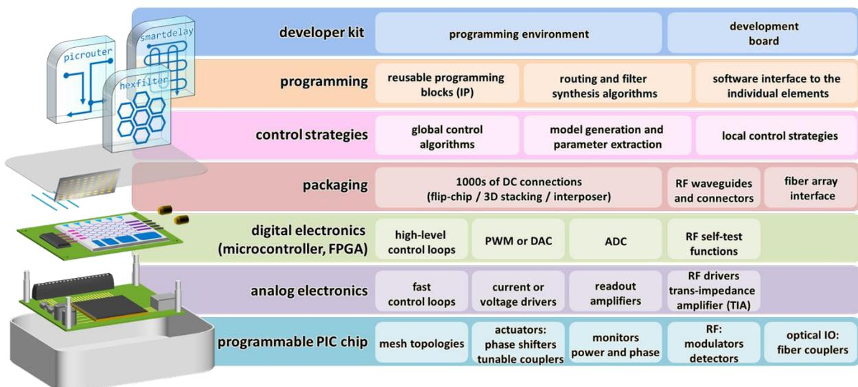
Fig. 2. Technology stack for programmable photonic circuits.
