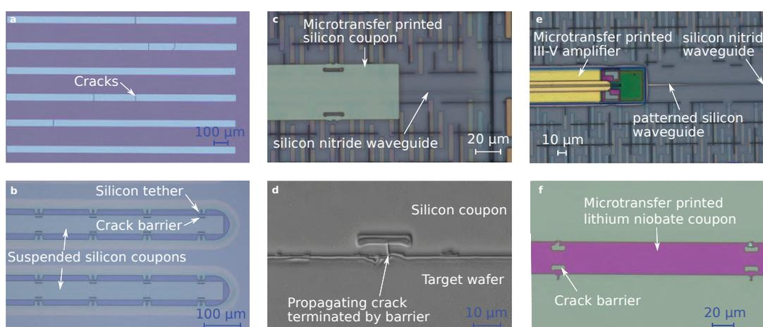
Fig. 1. Microscope pictures of microtransfer printed Si coupons without crack barriers (a), 400 nm thick suspended Si coupons with crack barriers on the source silicon-on-insulator wafer (b), a printed Si coupon in the recess of a Ligentec  $\text{Si}_3\text{N}_4$  die (c), effective crack termination by the crack barrier (d), printed SOA on top of a printed and patterned Si coupon (e), printed LN coupon (f).
