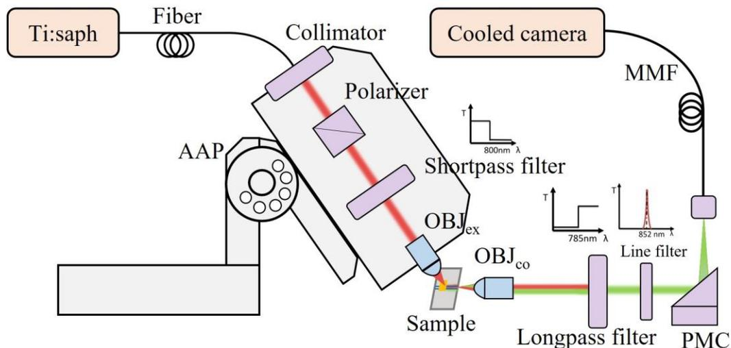
Figure 5. The schematic diagram of the free-space excitation experimental setup. Ti:saph: tunable Ti:sapphire laser, OBJex: objective (50 $\times$ , NA=0.6) for free-space excitation, AAP: adjustable angle plate, OBJco: objective (50 $\times$ , NA=0.65) for signal collection, PMC: parabolic mirror collimator, MMF: multimode fiber.
