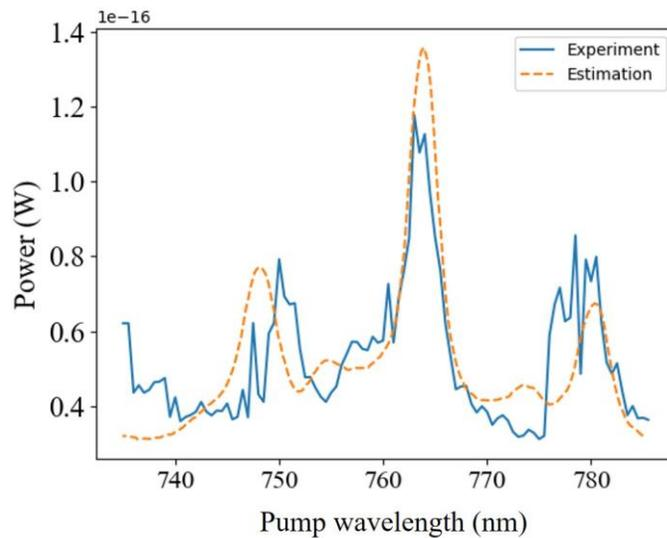
Figure 6. The signal power obtained through the cooled camera. The blue spectrum is the experimental result and the dashed spectrum is the estimated result.
