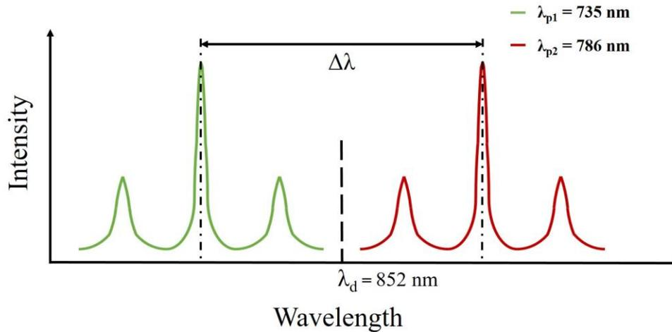
Figure 2. The Raman spectra with pump wavelengths of  $\lambda_{p1}$  nm and  $\lambda_{p2}$  produced by identical molecules.
