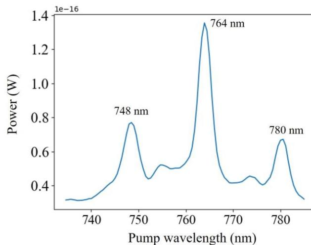
Figure 4. The estimated power of the light transmitting through the narrow band-pass filter at different pump wavelengths.
