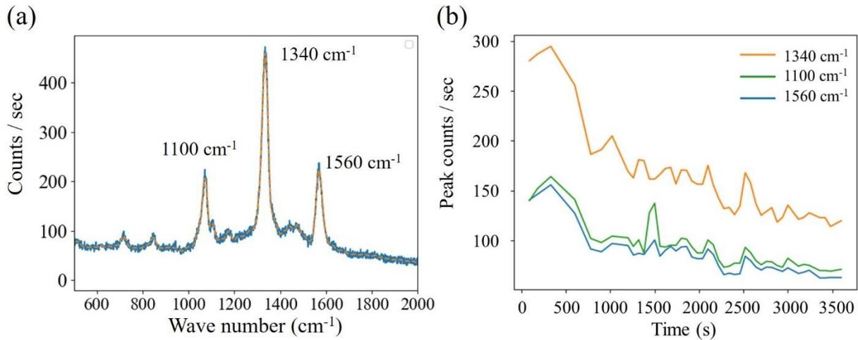
Figure 3. (a) The Raman spectra measured with CW laser light of 785 nm. (b) The count values of the Stokes peaks recorded under one-hour illumination.
