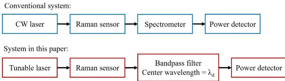
Figure 1. Flow diagrams of the conventional Raman detection system and the novel Raman detection system.
