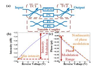
Fig. 1. (a) Schematic of the proposed configurable modulator circuit. PS: (static) phase shifter; PDM: plasma dispersion modulator; TC: tunable coupler. (b), (c) Intensity and phase response of a stand-alone PN modulator [4].
