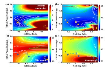
Fig. 2. Simulation of a PN modulator with a 0-6 V drive voltage. We sweep the coupling  $\kappa$  and the static phase shift  $\phi_s$ . (a) Spurious intensity modulation; (b) nonlinearity of the phase response; (c) minimal transmission (insertion loss); (d) phase modulation range. The green curve indicates the 'naked' PN modulator, without the circuit.
