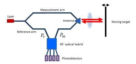
Figure 1: Schematic of a homodyne LDV
