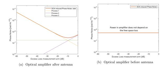
Figure 4: Plot of SOA phase noise as a function of the excess loss of the measurement arm when the SOA is in the measurement arm, assuming  $P_{ref} = 100 \mu W$ .
