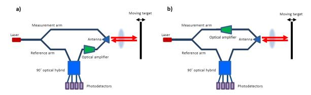
Figure 3: Optical amplifier in measurement arm; a) after antenna and b) before antenna
