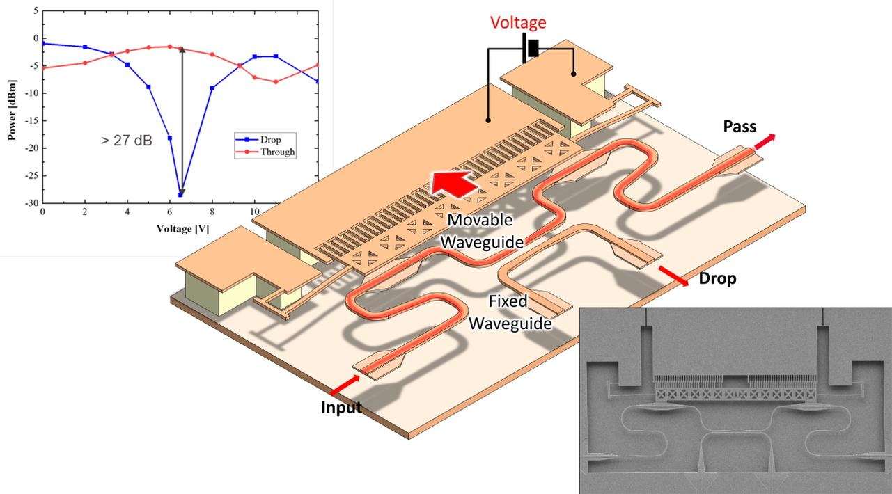
Figure 2. MEMS Tunable coupler implemented in the iSiPP50g process.<sup>13</sup> The light is coupled through a broadband directional coupler<sup>28</sup> where one side is attached to a lateral comb drive. By pulling the waveguides apart the operation can switch between bar state and cross state with 25 dB extinction ratio.
