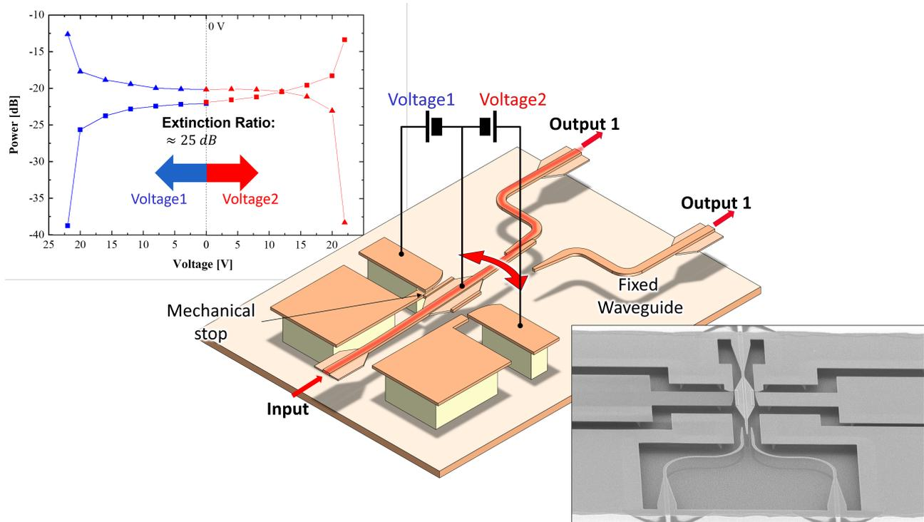
Figure 4. Compact single-pole double-throw MEMS switch implemented in the iSiPP50g platform.<sup>24</sup> The switch consists of a narrow suspended waveguide that can be pulled towards one of two side electrodes, coupling the narrow waveguide tip evanescently to the corresponding output waveguide.
