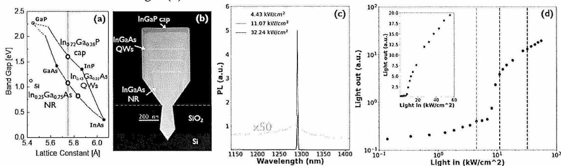
Fig. 1 (a) Bandgap energy (unstrained) vs. lattice constant, (b) Cross section of the InGaAs nano-ridge taken through HAADF STEM, (c) Spectra of the nano-ridge laser for different pump intensities, (d) light in-light out curve of the nano-ridge laser on logarithmic and linear (inset) scale with dashed lines referring to the pump intensities in the PL spectra.
