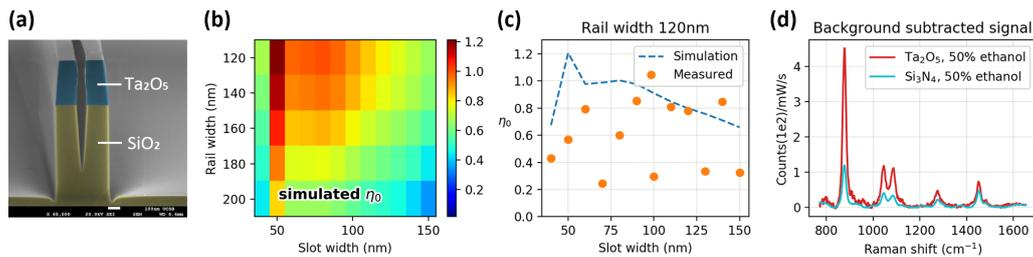
Figure 1: (a) Cross-section of a  $\text{Ta}_2\text{O}_5$  slot waveguide (b) Simulated  $\eta_0$  of slot waveguides with varied slot and rail widths (c) Simulated and measured  $\eta_0$  of waveguides with 120 nm wide rails (d) Raman spectra of 50% ethanol measured on the optimal  $\text{Ta}_2\text{O}_5$  and  $\text{Si}_3\text{N}_4$  slot waveguides.
